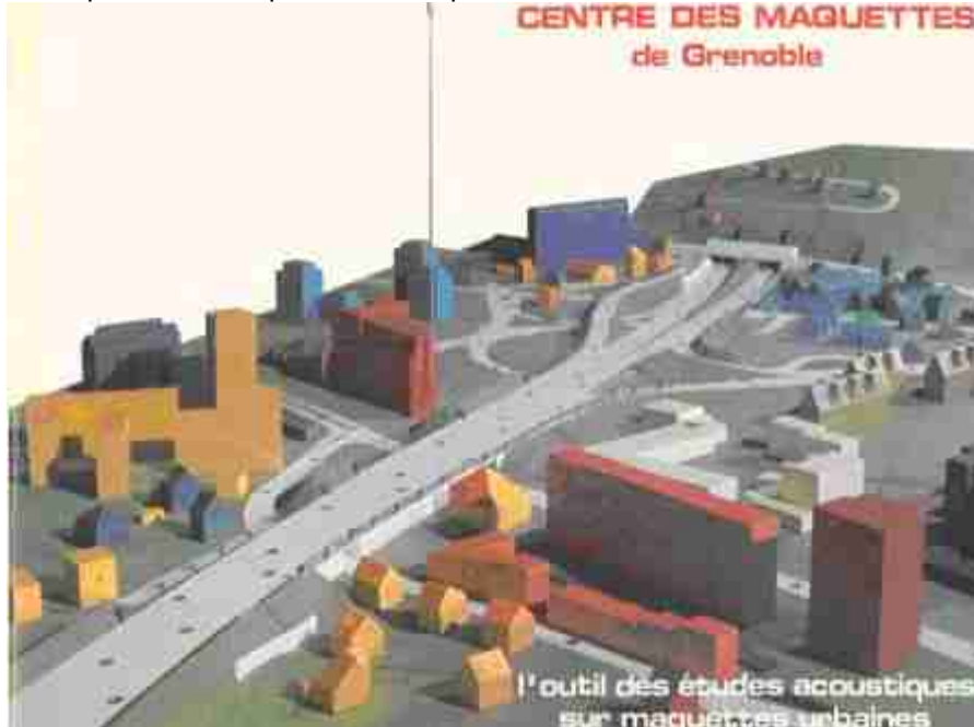
Figure 5: scale model studies for noise mapping (Centre des maquettes, Grenoble).
