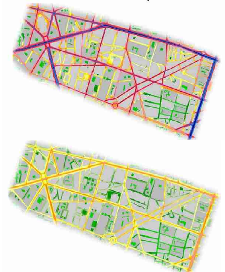
Figure 18: Action plan, simulation of noise levels on a normal working day and during the “No-cars today” operation (Journée sans voiture).
