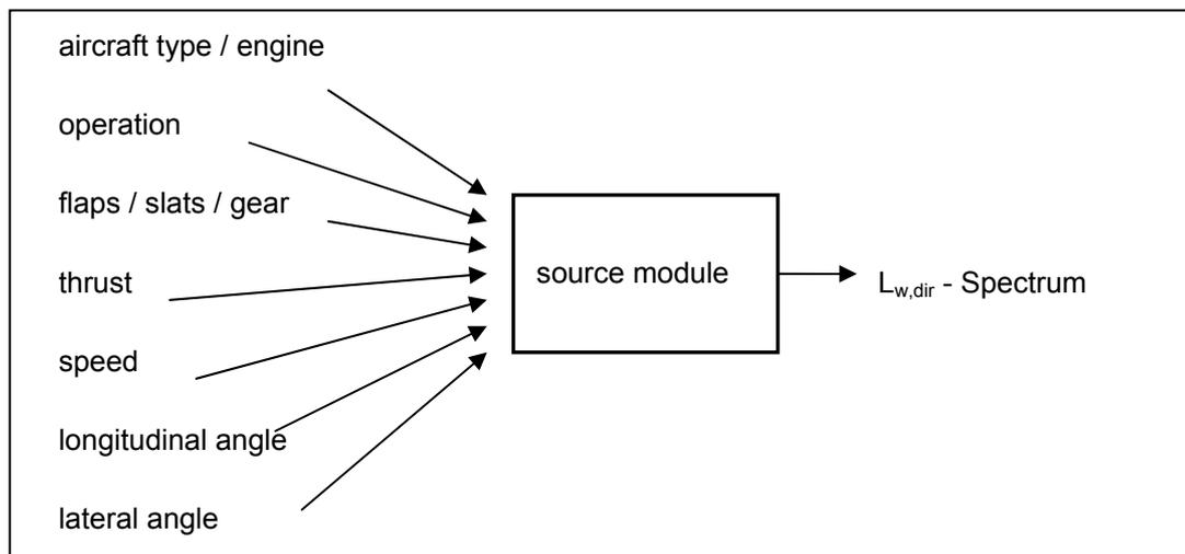
Figure 2-3 Possible input parameters for defining a specific source spectrum
