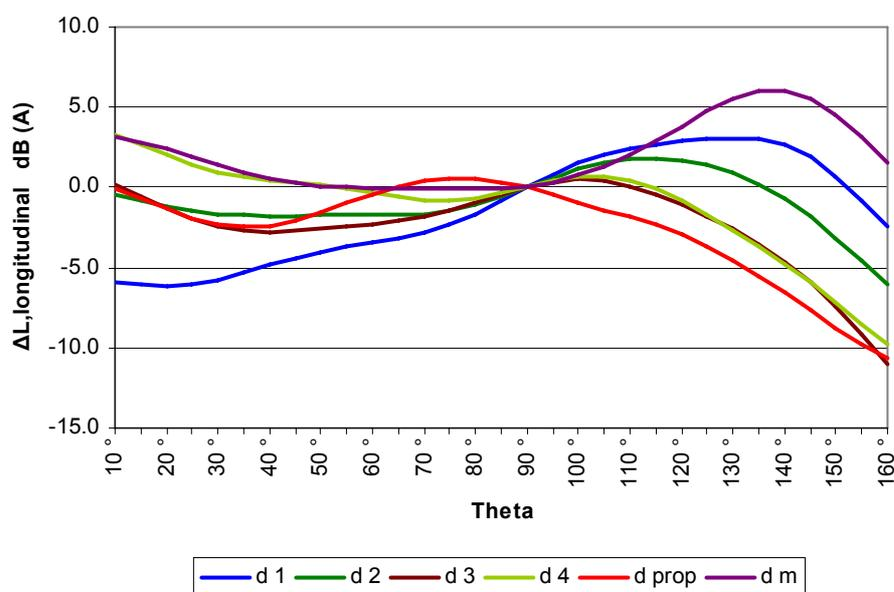
Figure 3-4: Six classes of longitudinal directivity for departures. Details see Annex A
