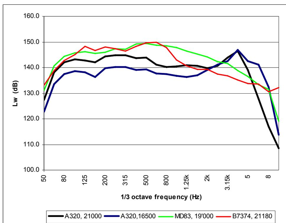
Figure C-1 Examples of sound power spectra (not A-weighted)
