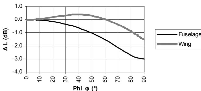
Figure 3-5 Installation effect for wing- and fuselage mounted engines
