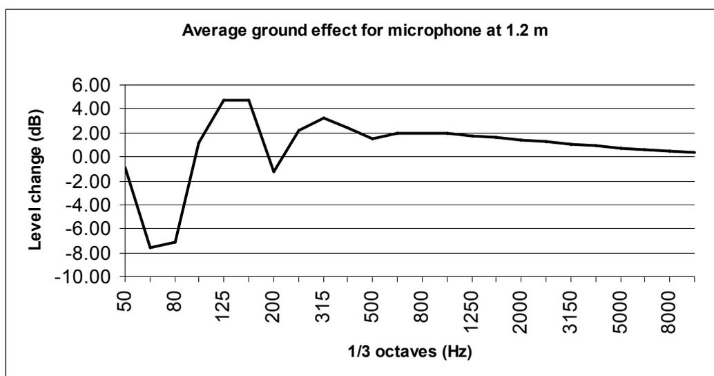
Figure 5-2 Ground effect of Table 5-1 (Parameters are described in the text)
