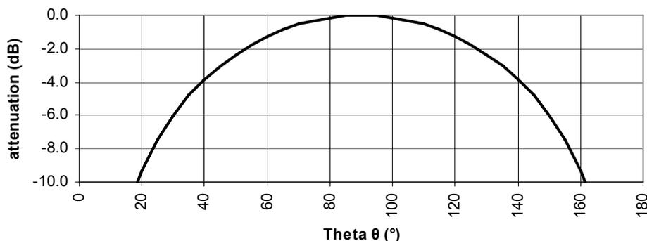
Figure 3-3 Spherical attenuation relative to shortest distance for a level flight [=  $20 \lg(\sin \theta)$ ]
