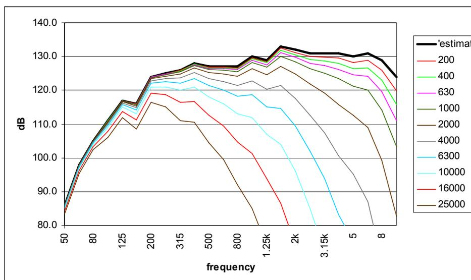
Figure 5-1 Example of A - weighted source spectrum ("estimat" =  $L_{pA}(1m)$ ) with added air absorption for various distances (in feet)
