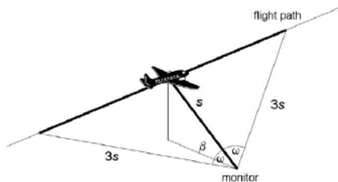
Figure 3-2: Maximum length of flight path for levels above  $L_{ASmax} - 10$  dB
