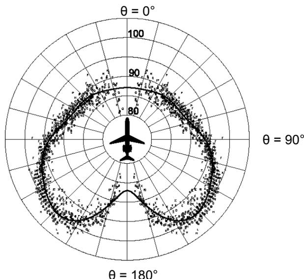
Figure 3-1: Example of longitudinal directivity. A-weighted levels from 14 measurements (taken at various lateral angles) for take-off of DC9-30. The plot shows the measured sound levels reduced to  $r = 305$  m as a function of the emission angle  $\theta$ . The fitted curve is used in FLULA [8].
