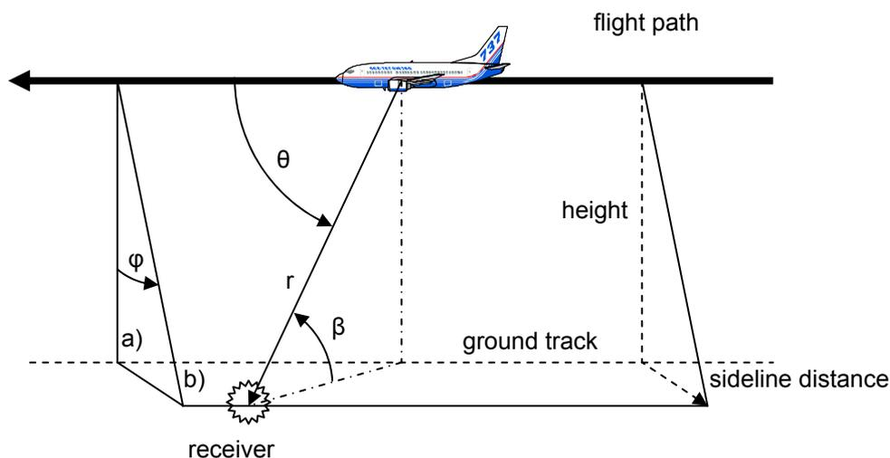
Figure 2-2 Aircraft sound emission co-ordinates theta ( $\theta$ ) and phi ( $\varphi$ ), and the ground referenced quantities: distance to the receiver  $r$  and elevation angle beta ( $\beta$ ) of sound incidence
