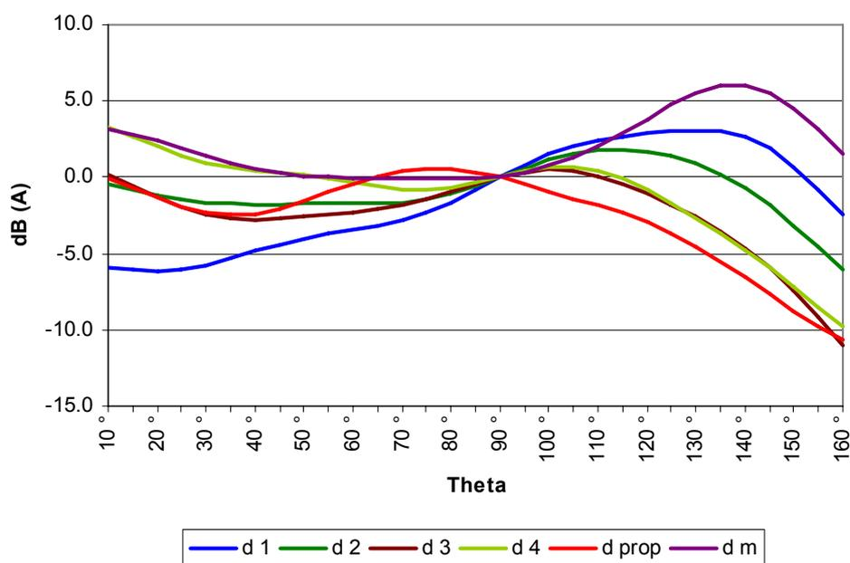
Figure A-1 Directivity functions for the A-level at constant distance of 305 m around the source
