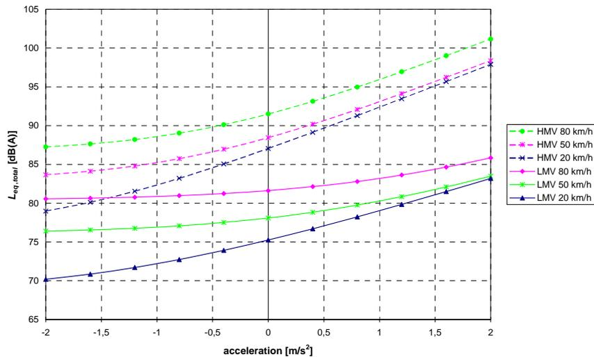
figure 19: Calculated  $L_{W,line,eq}$  as a function of the vehicle acceleration, for a single light or heavy motor vehicle at 20, 50 and 80 km/h
