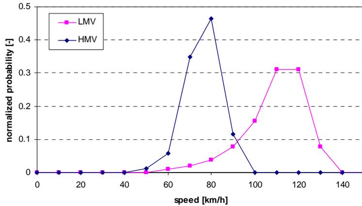
figure 6: Input speed distribution for motorway traffic situation
