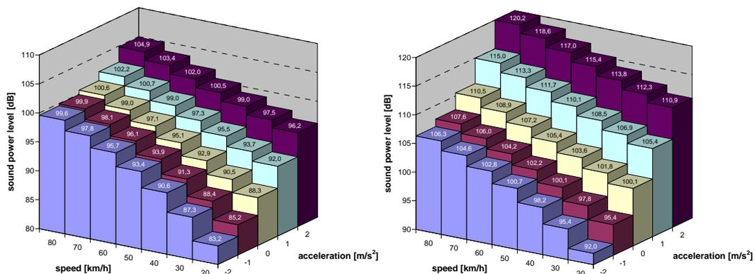
figure 3:  $L_w$  instantaneous sound source levels for a light motor vehicle (left) and heavy motor vehicle (right)
