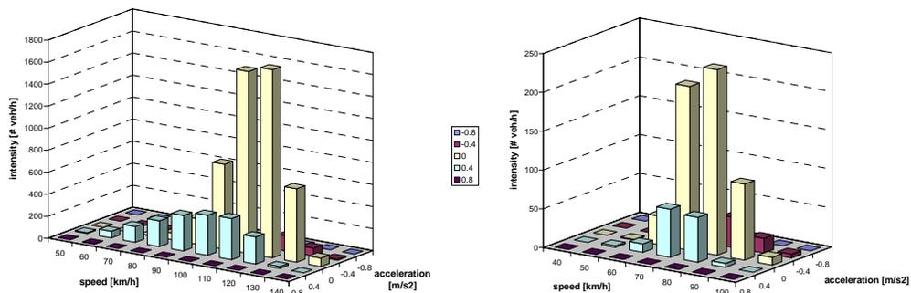
figure 7: Distributions of generated random vehicle speed and acceleration values for light motor vehicles (left) and heavy motor vehicles (right) on a motorway
