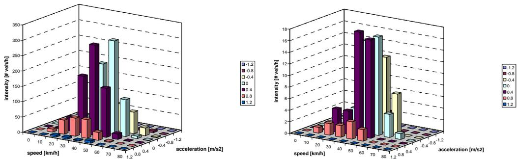
figure 9: Distributions of generated random vehicle speed and acceleration values for light motor vehicles (left) and heavy motor vehicles (right) on an urban 50 km/h road
