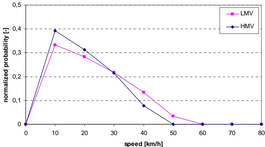
figure 11: Input speed distribution for intersection downstream traffic
