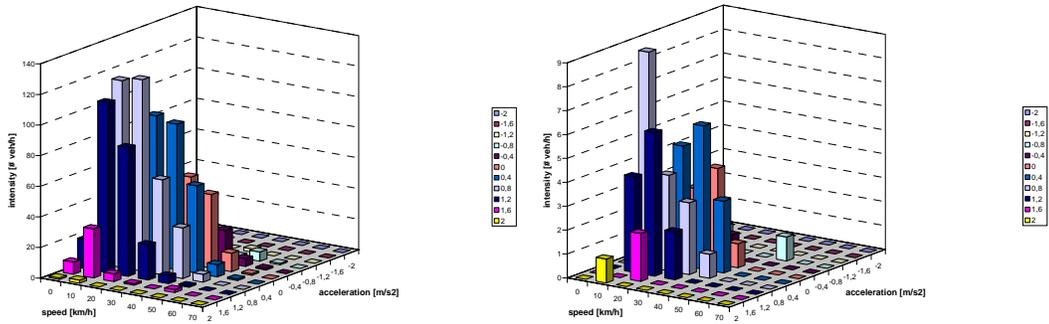
figure 12: Distributions of generated random vehicle speed and acceleration values for light motor vehicles (left) and heavy motor vehicles (right) downstream of an intersection
