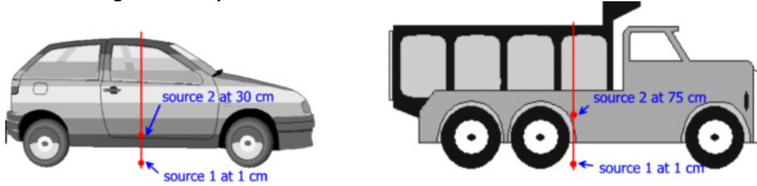
figure 2: Drawing of noise source positions
