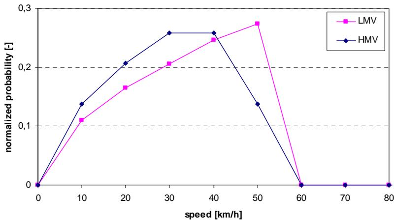
figure 13: Input speed distribution for intersection upstream decelerating traffic
