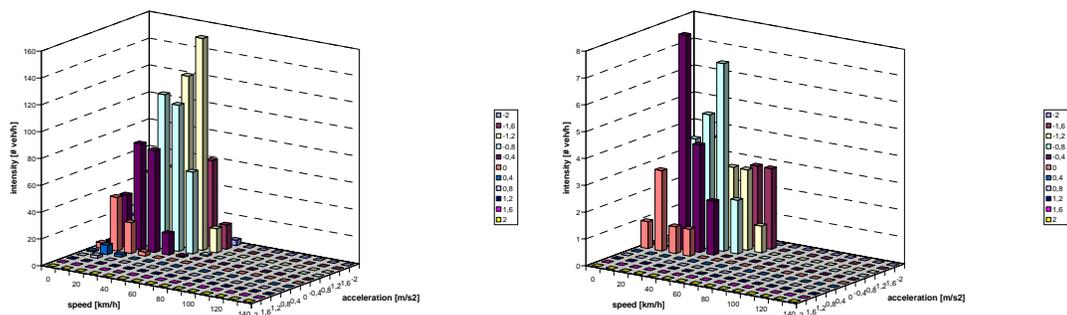
figure 14: Distributions of generated random vehicle speed and acceleration values for light motor vehicles (left) and heavy motor vehicles (right) upstream of an intersection
