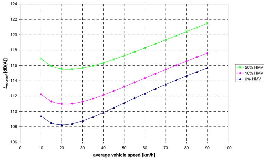
figure 17: Calculated  $L_{W,line,eq}$  as a function of the average vehicle speed, for a traffic intensity of 2000 veh/h with 0%, 10% and 50% heavy motor vehicles
