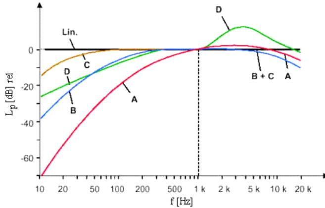
figure 1: Frequency weighting curves, showing the attenuation factor for each frequency
