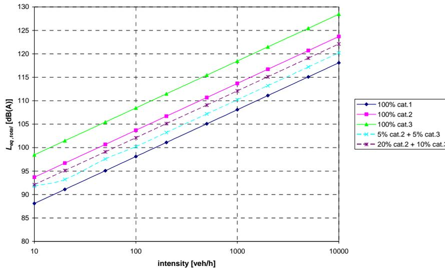
figure 15: Calculated  $L_{W,line,eq}$  as a function of traffic flow intensity, for various compositions of categories at 50 km/h and no acceleration
